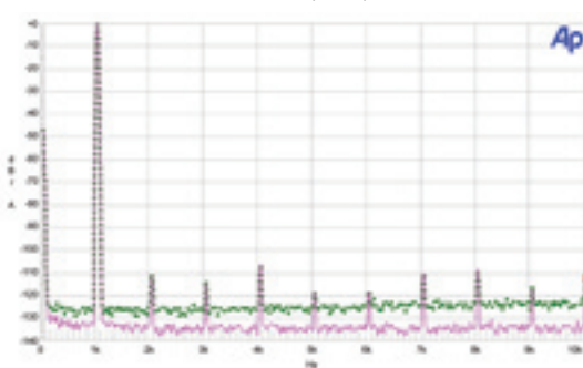
Naim DAC 1kHz: With Dither 24 bit (violet) and 16 bit Normal
